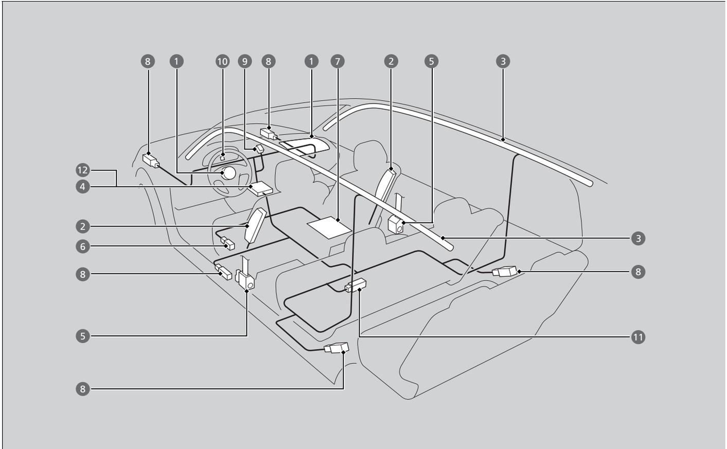
The front, side, and side curtain airbags are deployed according to the direction and severity of impact. Both side curtain airbags are deployed in a rollover. The airbag system includes:
