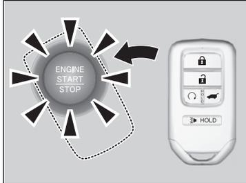
1. Touch the center of the **ENGINE START/STOP** button with the **H** logo on the keyless remote while the **ENGINE START/STOP** button is flashing. The buttons on the keyless remote should be facing you.
