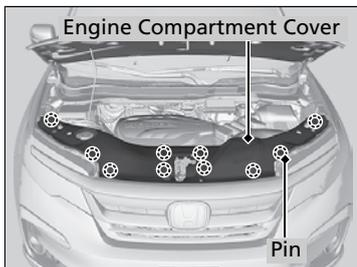
1. Pull up on the engine compartment cover, remove it from the pins.
