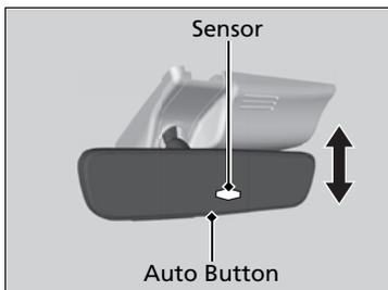
When you are driving after dark, the automatic dimming rearview mirror and power door mirror reduce the glare from headlights behind you. Press the AUTO button to turn this function on and off. When activated, the AUTO indicator comes on.
