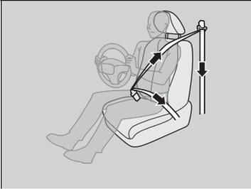
The front seats are equipped with automatic seat belt tensioners to enhance safety.
