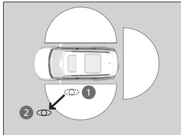
When you walk away from the vehicle with all doors and tailgate closed while carrying the keyless remote, the doors will automatically lock.
