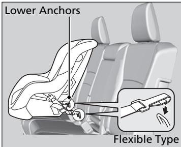
2. Place the child seat on the vehicle seat, then attach the child seat to the lower anchors according to the instructions that came with the child seat.
