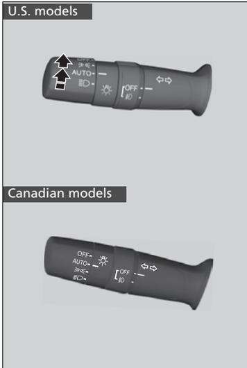
Automatic lighting control can be used when the power mode is in ON.
