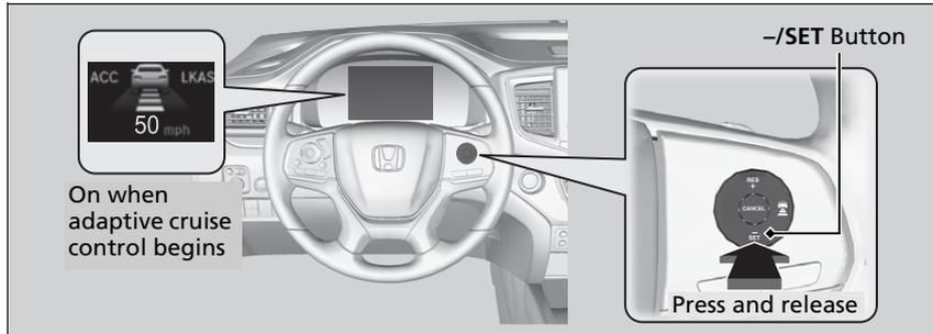
Take your foot off the pedal and press the **-/SET** button when you reach the desired speed. The moment you release the **-/SET** button, the set speed is fixed, and ACC begins.
