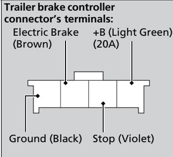
Have a qualified mechanic install your trailer brake controller following the trailer brake controller manufacturer's instructions. Failure to properly install the trailer brake controller may increase the distance it takes for you to stop your vehicle when towing a trailer.
