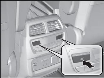
The power mode must be in ON to use the seat heaters.
