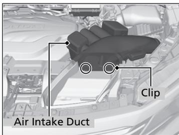
2. Remove the holding clips and the air intake duct.
