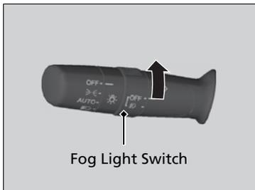
When the parking lights or the headlights are on, turn the fog light switch on to use the fog lights.
