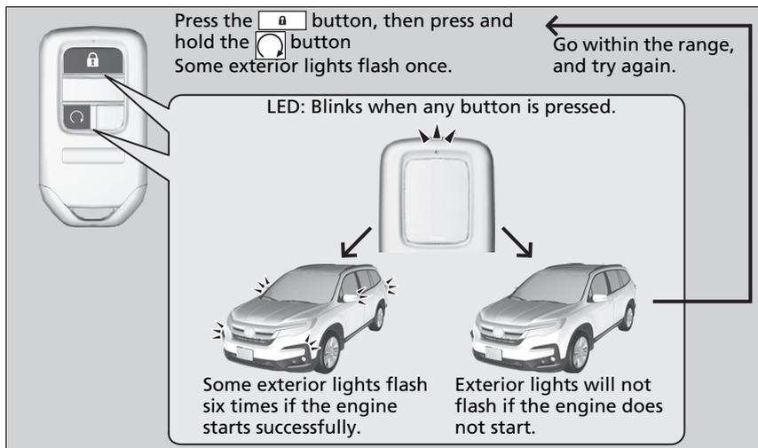
When started remotely, the engine automatically shuts off after 10 minutes of idling and/or the brake pedal and **ENGINE START/STOP** button have not been pressed simultaneously.
