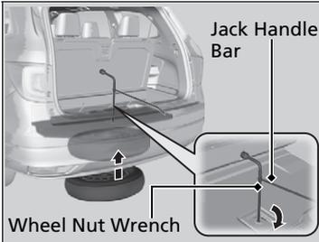
3. Slowly turn the wheel nut wrench clockwise to take up the hoist cable slack. Make sure the bracket is seated in the center hole of the flat tire.
