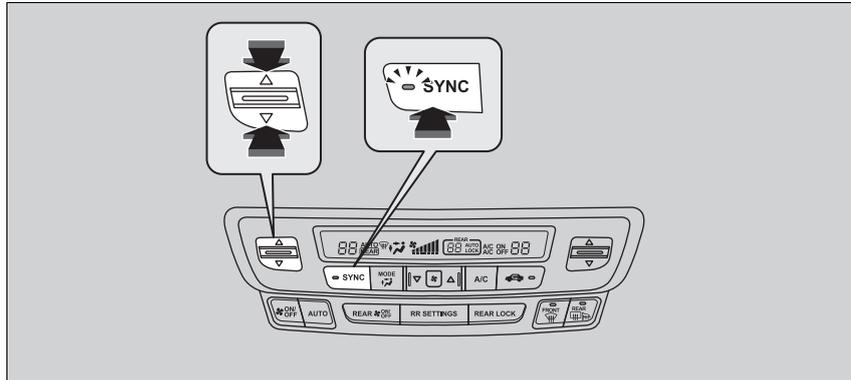
You can set the temperature synchronously for the driver side, front passenger side and rear seats in synchronization mode.
