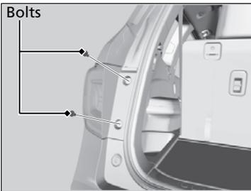
1. Use a Phillips-head screwdriver to remove the bolts.
