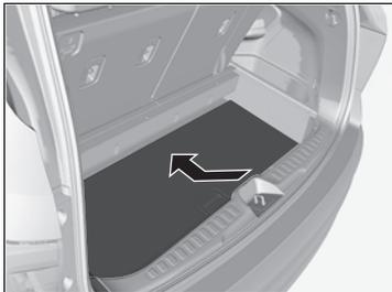
3. Push the far end of the lid down to the bottom of the under-floor storage area, then lower the other end.
