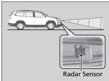
The radar sensor is located behind the emblem.
