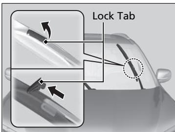
2. Place a cloth on the edge of the lock tab. Push the lock tab up with a flat-tip screw driver.
