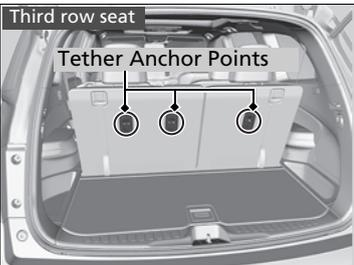
A tether anchor point is provided behind each second and third row seating position. If you have a child seat that comes with a tether but can be installed with a seat belt, the tether may be used for additional security.
