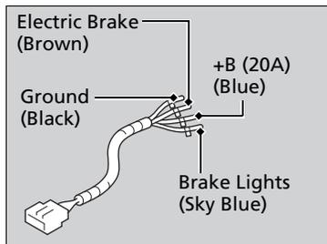
The trailer hitch harness is used to install the controller for the electric trailer brakes. Insert the trailer brake fuse into the engine compartment sub fuse box.
