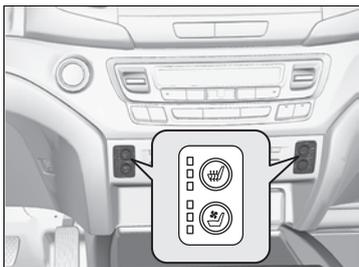
Press the seat heater or the seat ventilator button:
