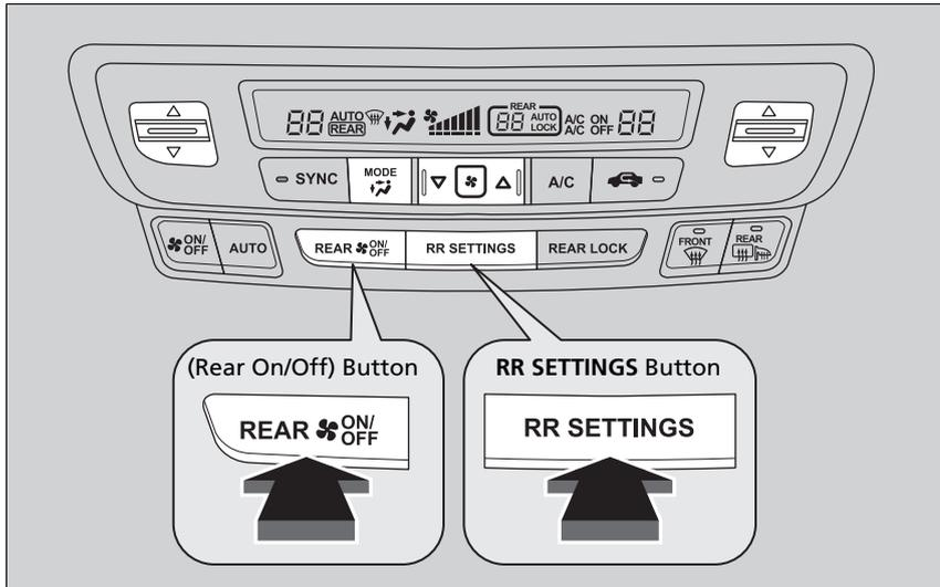
Use the system when the engine is running and the climate control system is operating.
