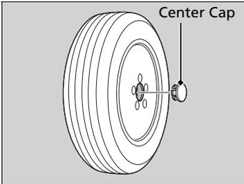
1. Remove the center cap and place the flat tire face up under the hoist.
