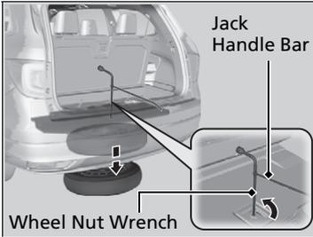
**5.** Put the wheel nut wrench with the jack handle bar on the hoist shaft. Turn the wrench to the left to lower the spare tire to the ground.
