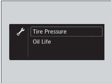
Shows the current condition of the tire pressure and the remaining oil life.
