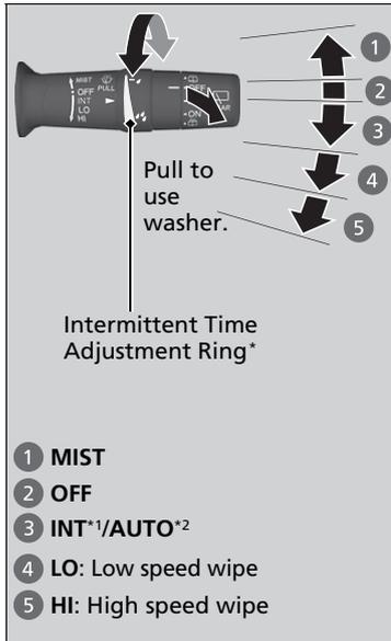
The windshield wipers and washers can be used when the power mode is in ON.
