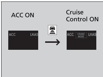
Press and hold the
