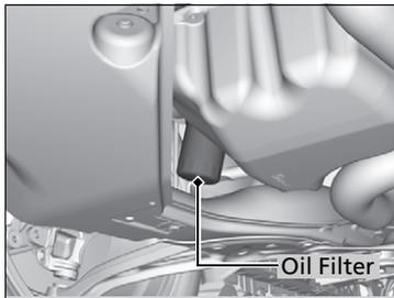
4. Remove the oil filter and dispose of the remaining oil.
